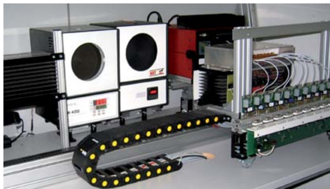
Automated calibration stations at Optris GmbH
